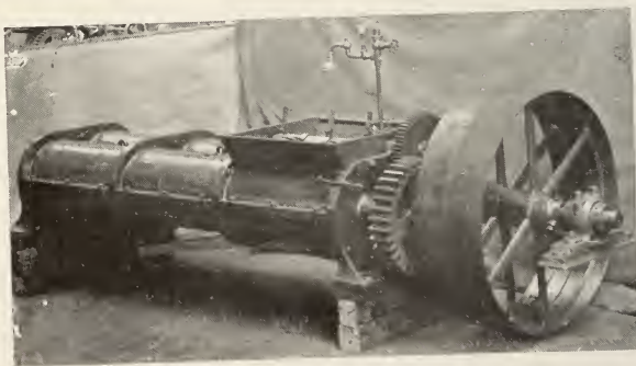
Three Segment Pulping Engine—Trough 800 and 2,000 lbs.
